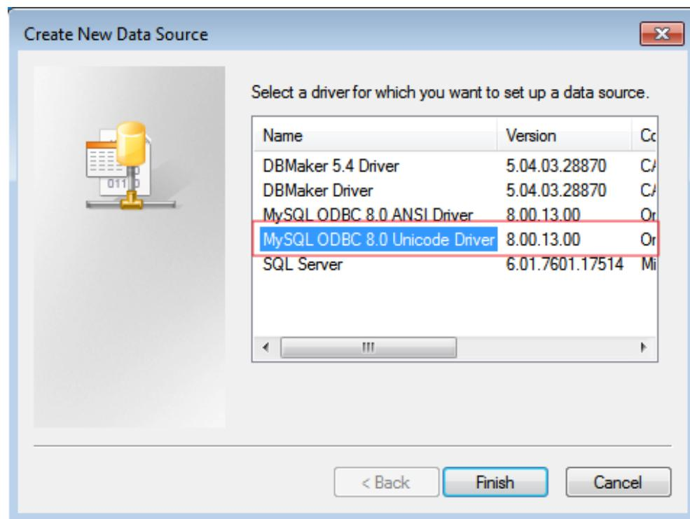
**Note:** Because DBMaker Java client uses Unicode encoding, the data source driver must select the MySQL ODBC 8.0 Unicode driver.
