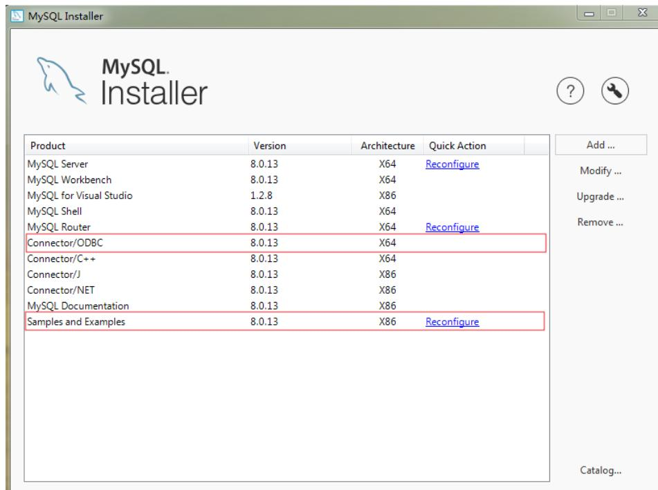
**Note:** Ensure that Connector/ODBC and Samples and Examples are installed
